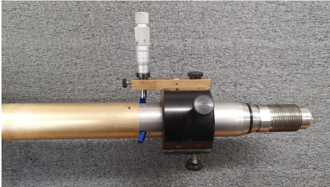
Figure 14: A micrometer set up on an RPM, used for calibrating the strain gauge transducers for measuring displacement
