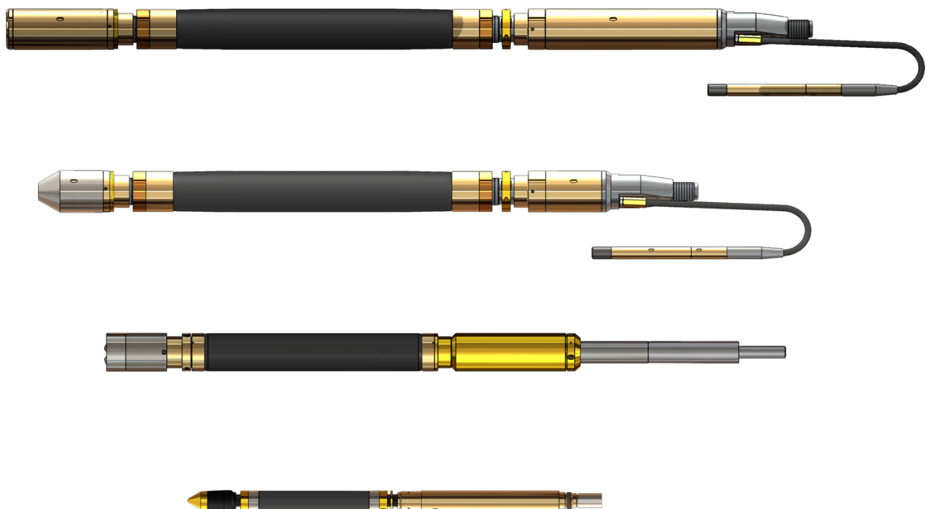
Figure 4. Rendered CAD images of some radial displacement pressuremeters. From top to bottom; 95HPD, 95HPD (Short), SBPM, RPM. Photo by Cambridge Insitu Ltd, 2022
