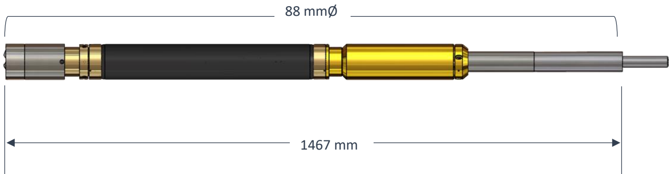
Figure 1.0. CAD render of an 88mm SBP configured without subs or rods.
