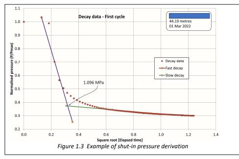
7. Note that the shut-in stresses are normalised by the maximum pressure (in effect  $P_R$ ) at the start of the fracture closure process. The horizontal axis is square root elapsed time, giving greater emphasis to the focal point of the closure response.
