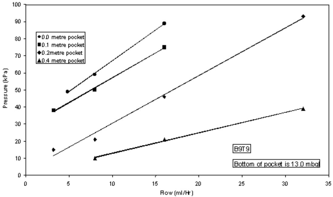
Fig. 3 Flow versus Pressure, selected data
