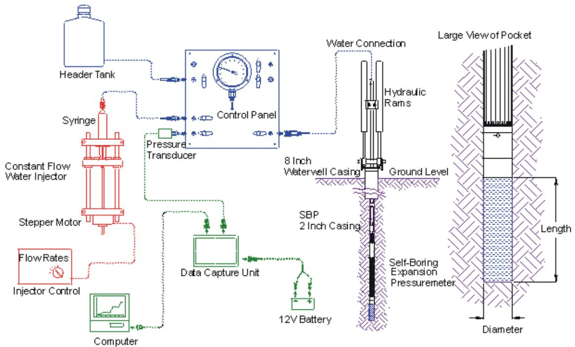
Fig. 1 The layout of the permeameter trial using a standard SBP
