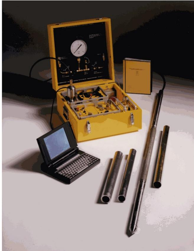
*Fig. 4 The Cone Pressuremeter*
