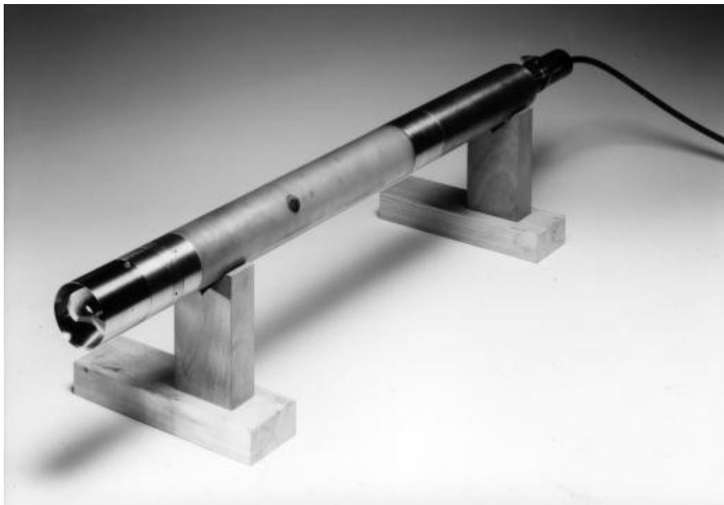
*Fig. 1 A Cambridge Self Boring Pressuremeter*
